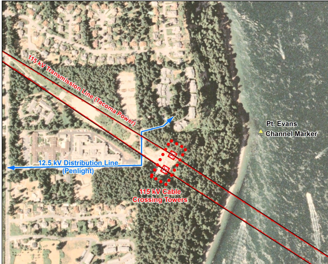
Figure 2.14 – Interconnection infrastructure near Point Evans, Tacoma Narrows
