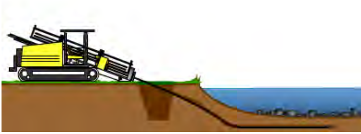
Figure 3.1- Horizontal directional drilling (HDD) rig
