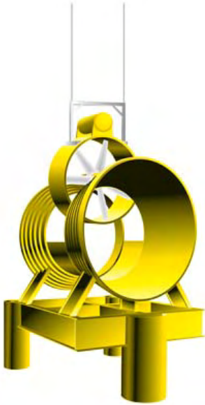
Figure 3.9 – Lunar RTT cassette deployment/recovery (Source: Lunar Energy) Note: the foundation and support structure shown have been superseded by the design in Figure 3.7.
