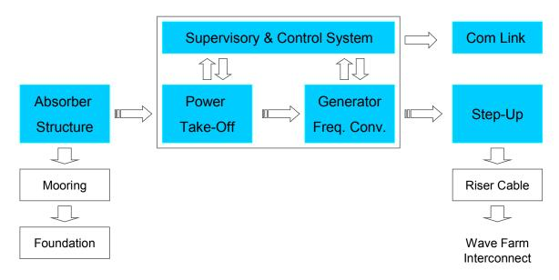
The following chart shows the likely electrical setup of the system. This design concept might change based on local site conditions and/or choice of technology.
