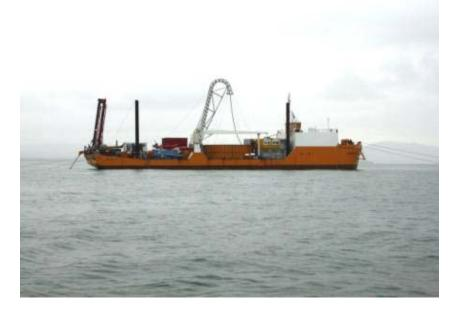
Illustration: Cable laying vessel
