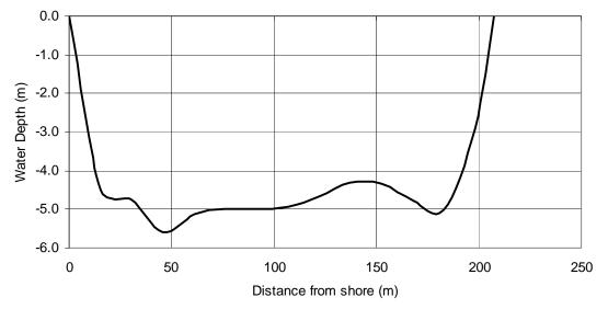
Figure 7: USGS Measurement Cross Section, showing water depth at a discharge rate of 63,900 ft^3/s
