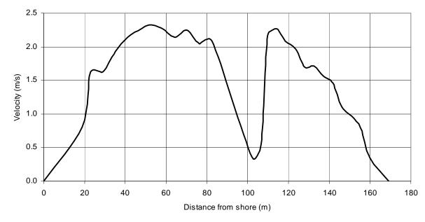
Figure 26: USGS cross-section showing velocity at a discharge rate of 41,200ft<sup>3</sup>/s
