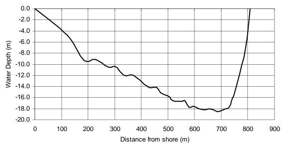
Figure 50: USGS cross-section showing water at a discharge rate of 219,000ft<sup>3</sup>/s
