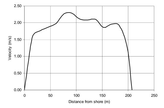
Figure 6: USGS Measurement Cross Section, velocity at a discharge rate of 63,900 ft^3/s
