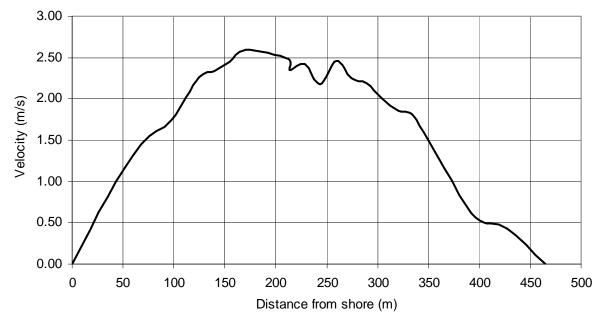
Figure 39: USGS cross-section showing velocity at a discharge rate of 183,000ft<sup>3</sup>/s
