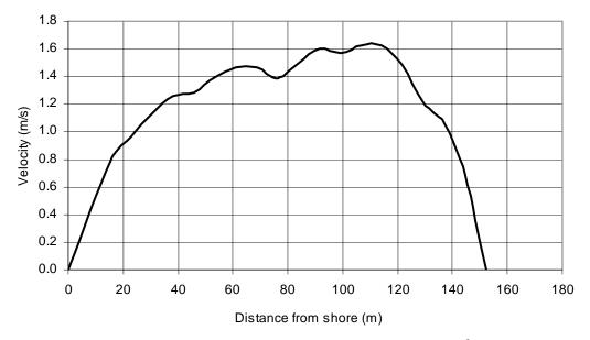
Figure 60: USGS cross-section showing velocity at a discharge rate of 17,200ft<sup>3</sup>/s
