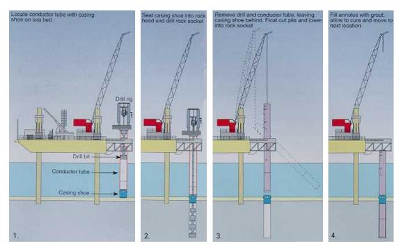
Figure 39 – Pile Installed in Bedrock (Seacore)
