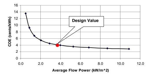
Figure 53 – Sensitivity of COE to average flow power in  $kW/m^2$
