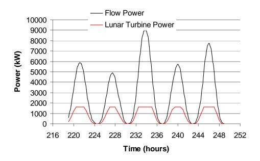
Figure 25 – Variation of flow power and electrical power output at the site
