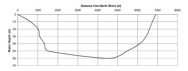
Figure 18 - Cape Blomidon channel cross section
