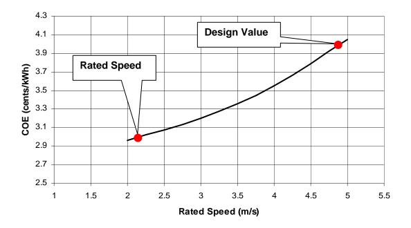
Figure 55 - Sensitivity of COE to design speed
