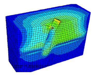
Figure 37 - Simulation of pile-soil interaction subject to lateral load (Source: Danish Geotechnical Institute)
