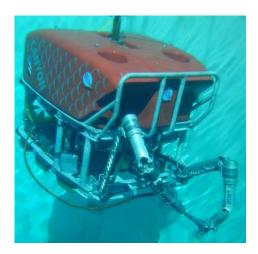
Figure 29 – Remotely Operated Vehicle (ROV) – (courtesy of Schilling Robotics - <u>www.ssaalliance.com</u>)
