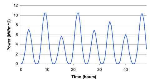
Figure 12 - Depth averaged power density variation at Cape Sharp over 48 hours
