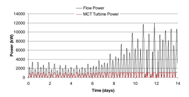
Figure 34 - Device power vs. flow power in cross sectional area of device
