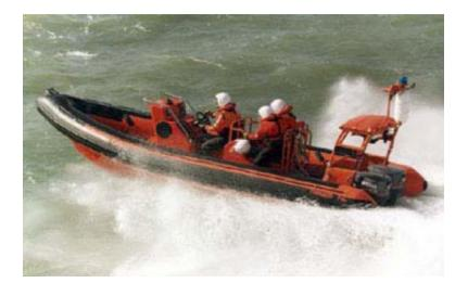
Figure 41: Typical Rigid Inflatable Boat (RIB)
