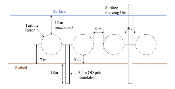
Figure 47 – MCT SeaGen Turbine Spacing Assumptions
