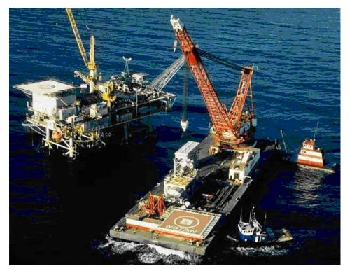
Figure 40 - 600 ton Derrick Barge WOTAN operating offshore (Manson Construction)
