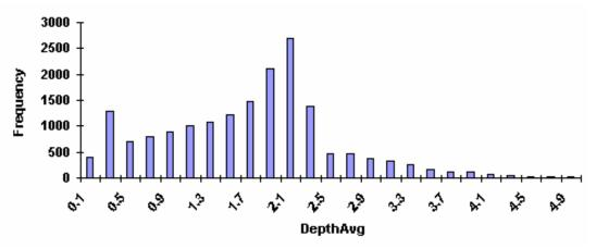
Figure 10 - Depth averaged velocity distribution at the Cape Sharp commercial site. Velocity shown is in m/s
