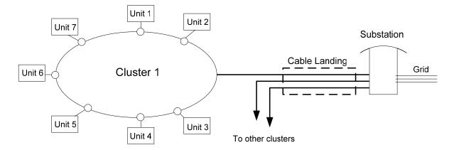
Figure 44 - Electrical Power Collection and Grid Interconnection for commercial plant
