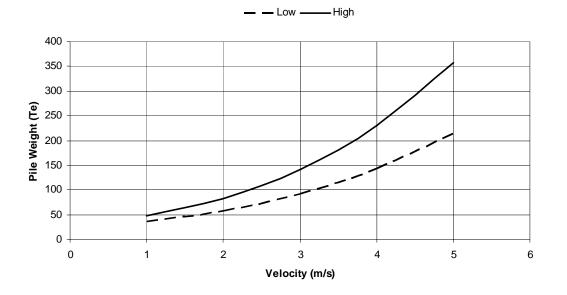
Figure 38 - Pile Weight as a function of design velocity for different sediment types
