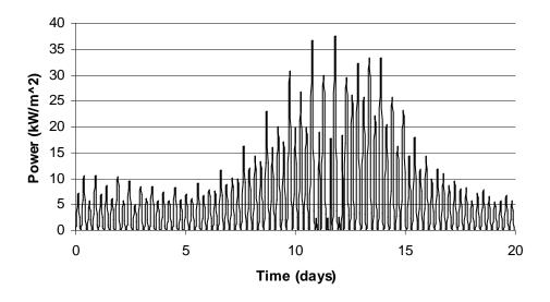
Figure 13 - Depth average power density at Cape Sharp
