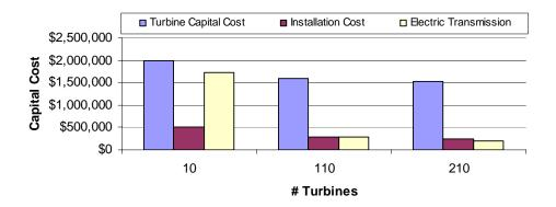
Figure 50 – Sensitivity of capital cost elements to number of installed turbines
