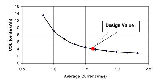
Figure 54 – Sensitivity of COE to average current speed (m/s) Clearly, the average velocity at the site has a significant effect on cost of energy, particularly if average current speeds are lower than expected. Note that these results are dependent on the shape of the velocity distribution histogram and therefore, we can not broadly draw conclusions about the cost of energy at other sites from this analysis (though
