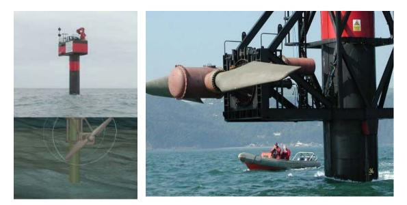
Operation Maintenance Figure 31 – MCT SeaFlow Test Unit (courtesy of MCT) (In printed from,' the pictures are upside down courtesy of Microsoft or our MS Word skills)
