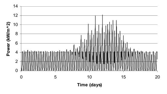
Figure 7 - Depth averaged power density at Cape Blomidon Transect over a full lunar cycle
