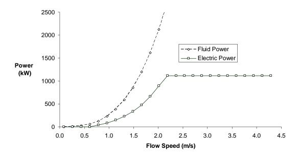
Figure 32 – Comparison of water current speed and electrical power output
