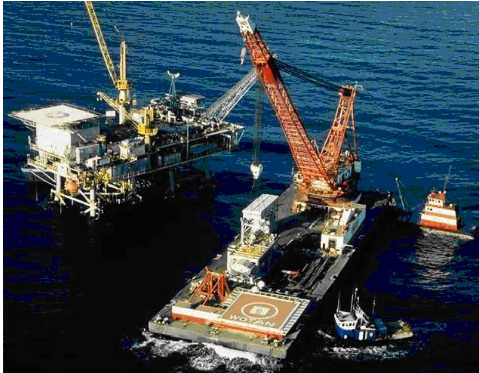
Figure 22 - Manson Construction 600 ton Derrick Barge WOTAN operating offshore (courtesy of Manson Construction)
