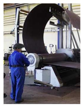
**Figure 9: Manufacturing Steel Tubular Sections**
