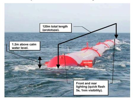
Figure 5: Pelamis pre-production prototype undergoing sea-trials
