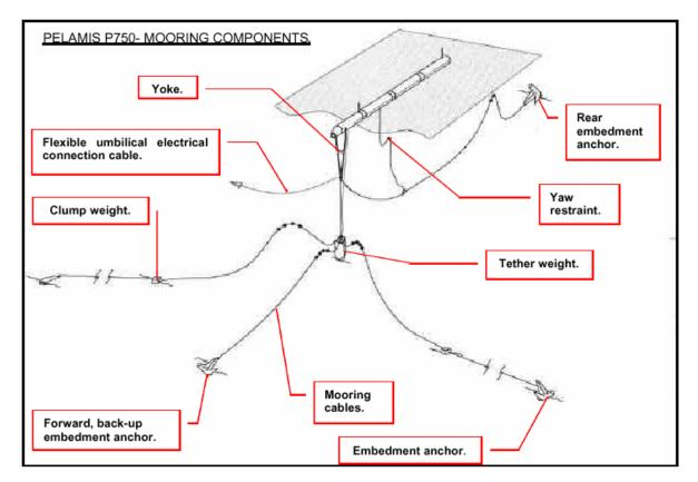
**Figure 10: Mooring Arrangement of Pelamis**
