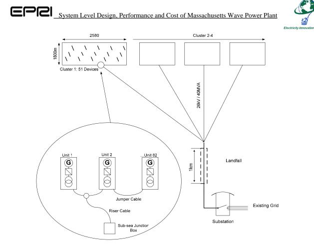
Figure 17: Overall System Layout and Electrical Connections
