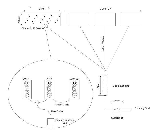
Figure 19: Overall System Layout and Electrical Connections
