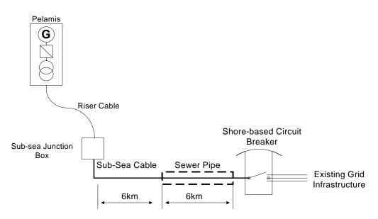
Figure 18: Electrical Interconnection of a Single Pelamis Plant
