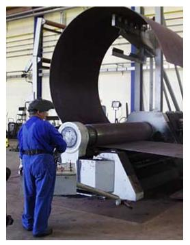
Figure 11: Manufacturing Steel Tubular Sections
