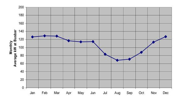
Figure 20: Monthly average power delivered to bus bar - Single Unit Pelamis Plant
