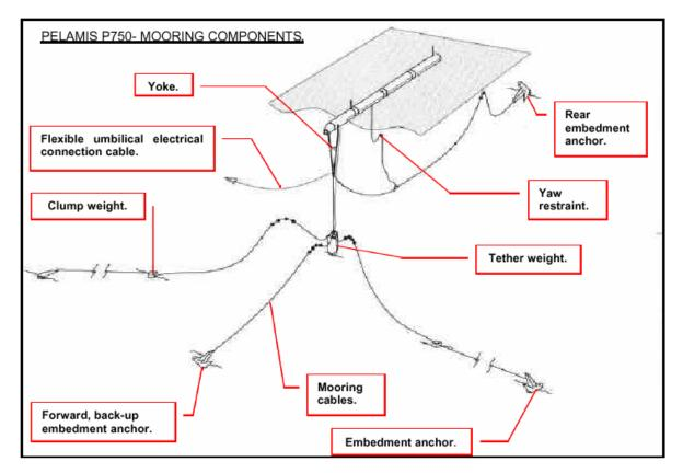
**Figure 12: Mooring Arrangement of Pelamis**
