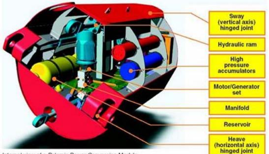
Internal view of a Pelamis Power Conversion Module.
