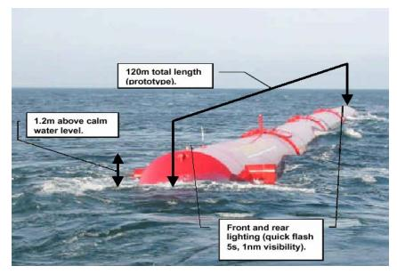
Figure 7: Pelamis pre-production prototype undergoing sea-trials
