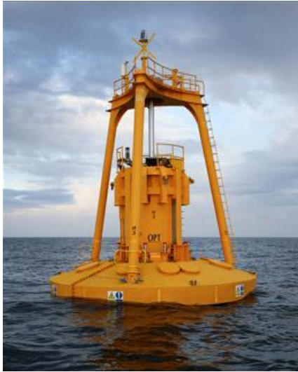
Figure 10 – OPT PB150 Power Buoy (Source: Ocean Power Technologies)
