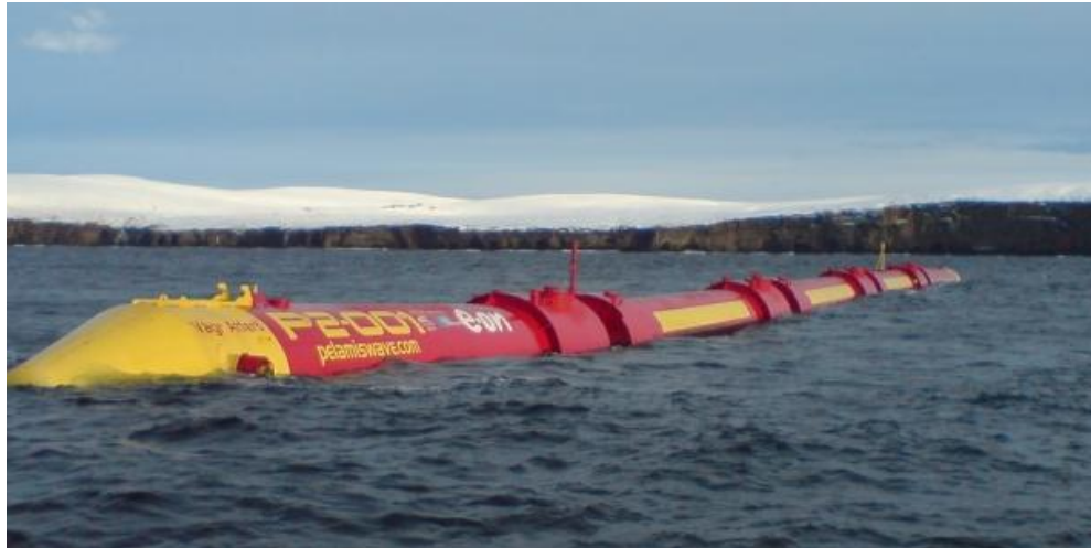
Figure 5 - Pelamis wave power device (Source: Pelamis Wave Power)
